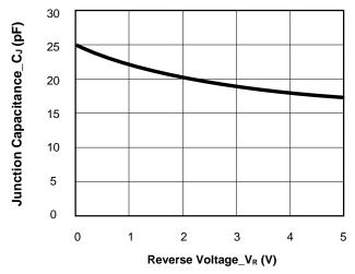
Junction Capacitance vs. Reverse Voltage
