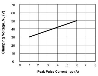
Clamping Voltage vs. Peak Pulse Current
